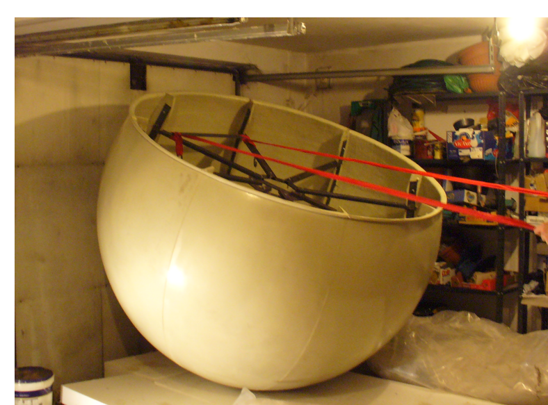
Prototype of the spherical shaped sun tracking device. To be developed in Bio-Eco-Matic Project
