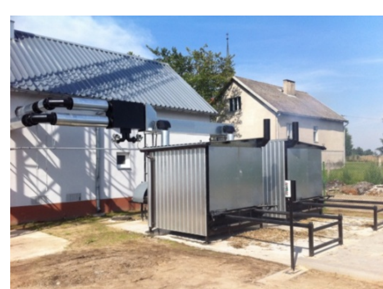
Prototype of the biomass drying system - to be developed in Bio-Eco-Matic Project
