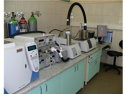
STA-QMS-FTIR Netzsch 409PG
