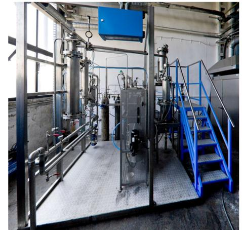
Experimental facility for studing pressurised fluidised oxy-fuel combustion and gasification of coal (1,6 MPa, 900°C, 2kg/h)
