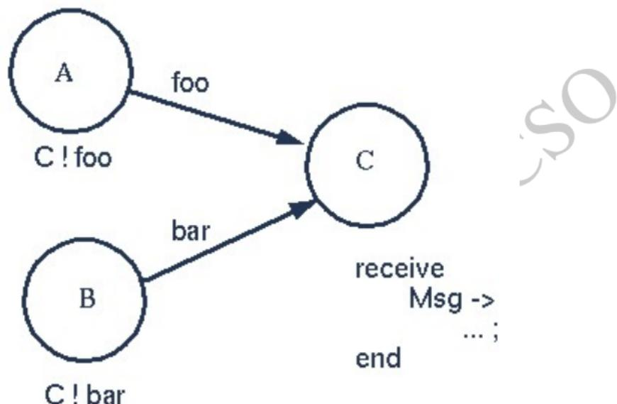
The first message to arrive at the process C will be processed - the variable `Msg` in the process C will be bound to one of the atoms `foo` or `bar` depending on which arrives first.
