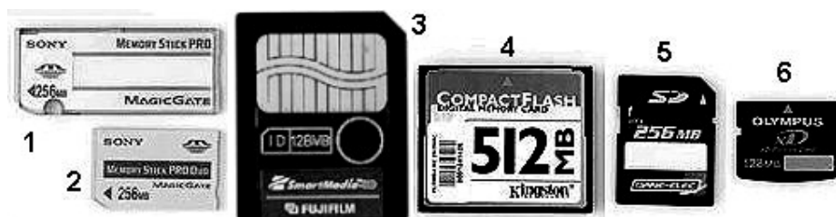
Rys. 3.11. Niektóre karty pamięci typu "flash": 1) MS - Memory Stick [50mm×21.5mm×2.8mm], 2) MSD - Memory Stick Duo [31×20×1.6], 3) SM - Smart Media [45×37×0.76], 4) CF - Compact Flash [43×36×3.3], 5) SD - Secure Digital [32×24×2.1], 6) xD Picture [20×25×1.7]
