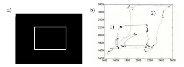
Fig. 1 a) Calibration contour and b) eyeball traces: 1) -well-calibrated, 2) ill-calibrated
