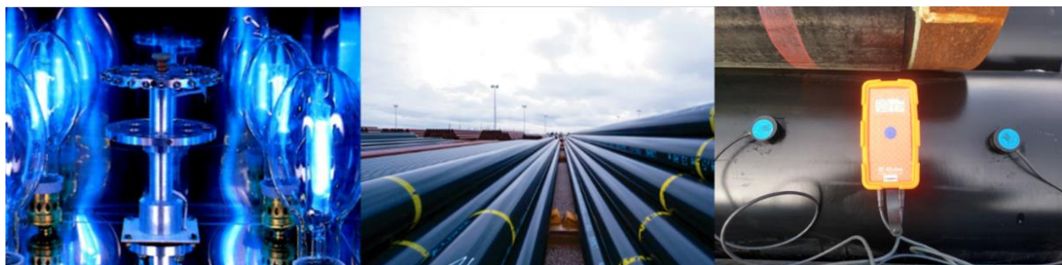
Figure 1: Artificial (left) and natural (middle) ageing of polyethylene. EIS measurement with the CQM probe (right).
